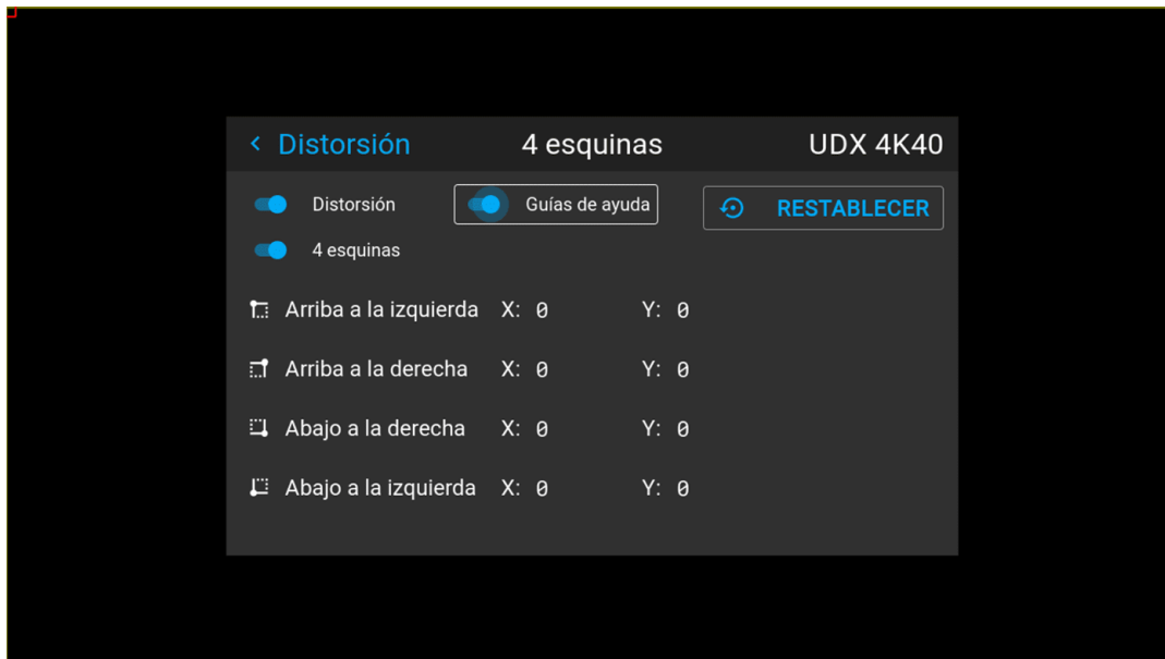
Imagen 9-35 Example of 4 corners warping menu, with helper lines active on the edges of the screen
